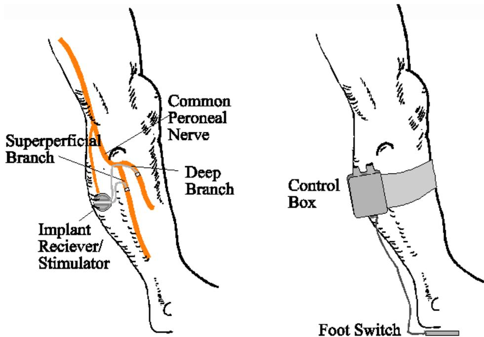
**Figure 6.** A two-channel implantable peroneal nerve stimulator (STIMuSTEP) allows individual stimulation of the deep and superficial branches of the common peroneal nerve for ankle dorsiflexion and eversion-inversion balance. (Courtesy of the Department of Medical Physics and Biomedical Engineering, Salisbury District Hospital, Salisbury, UK)
