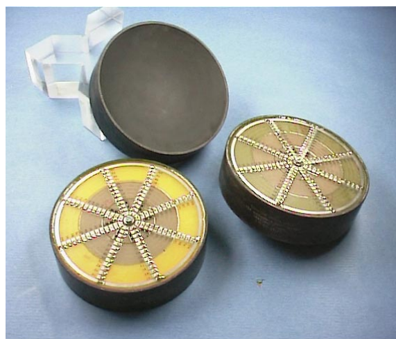
Fig.5 : 104 elements high power MRI compatible transducers
